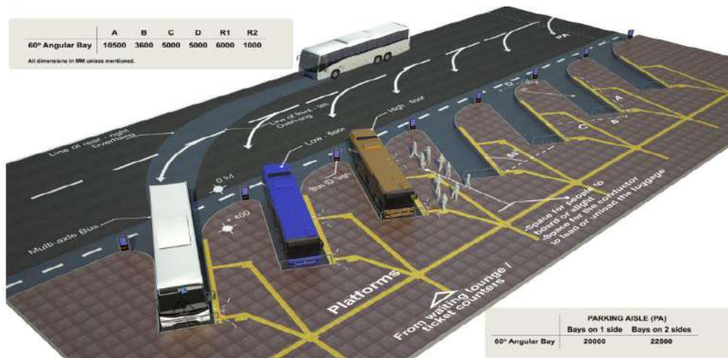
Figure 6-3: Passenger Boarding/Alighting Bay Options- Angular 60° Bay
