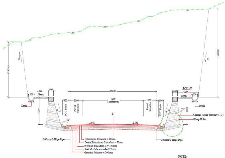
Type - 4- Typical Cross-Section For Two Lane Carriageway With Paved Shoulder
