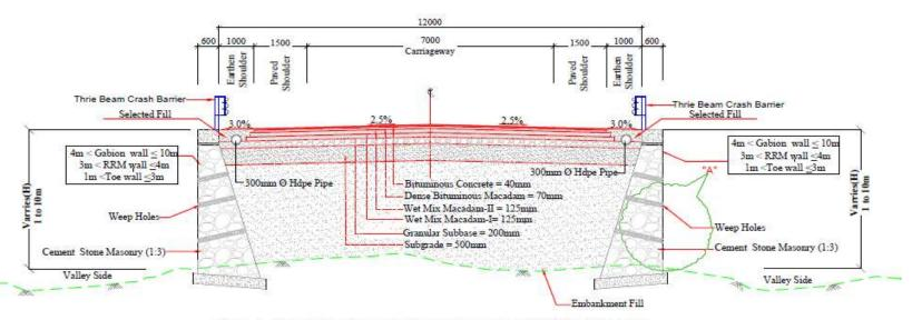
Type - 1 - Typical Cross-Section For Two Lane Carriageway With Paved Shoulder
