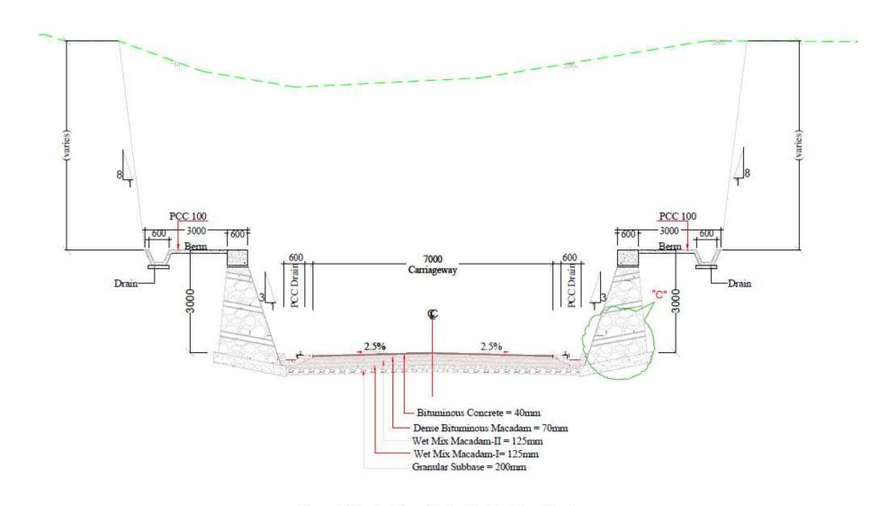
Type - C- Typical Cross-Section For Two Lane Carriageway
