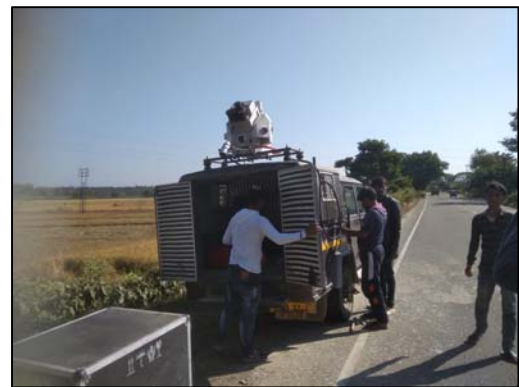
Mobile LiDAR used for the Project
