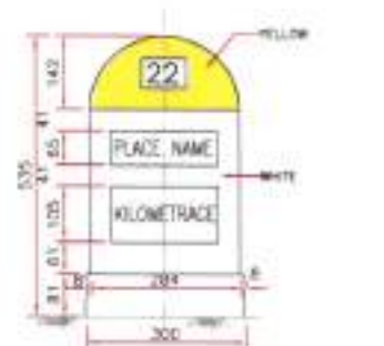
DETAIL OF FIFTH KILOMETRE STONE (SCALE 1:20)
