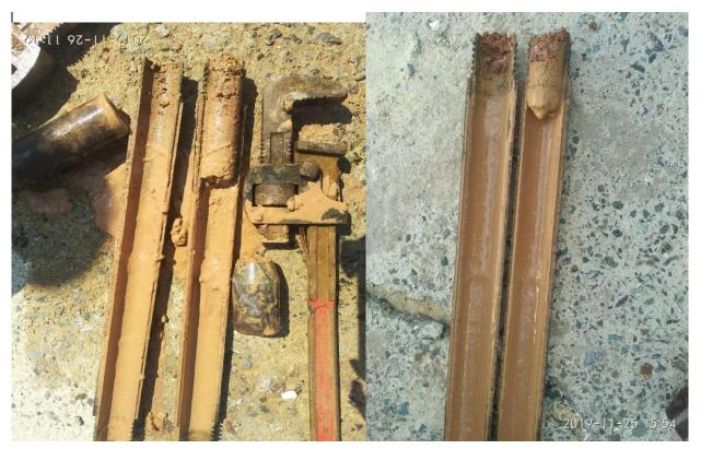
Fig.3. Soil Sample collected in SPT Sampler
