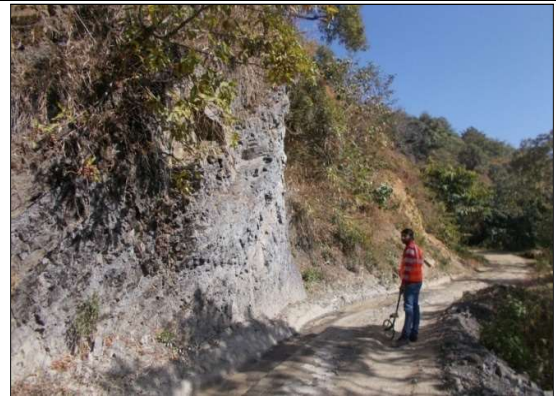
Chaining with Roadometer
