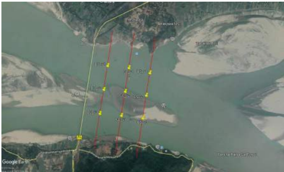
Figure 2.2: Location of Velocity Measurements and Cross-section
