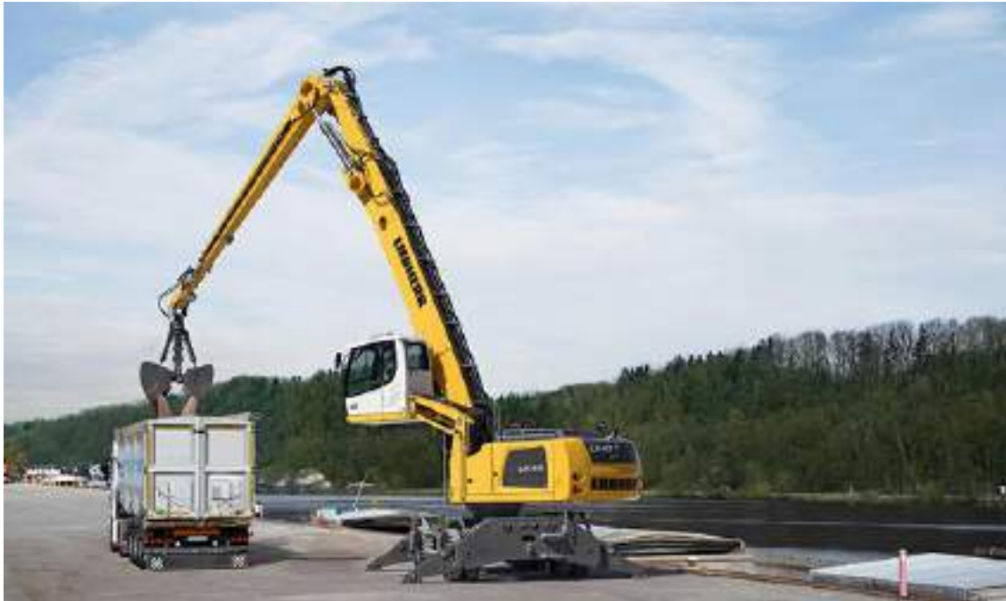
Figure 7.8: Typical General Purpose Mobile Harbour Crane
