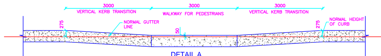
DETAIL A KERB DROP ON MEDIAN ALONG MAIN CARRIAGEWAY SCALE 1:50
