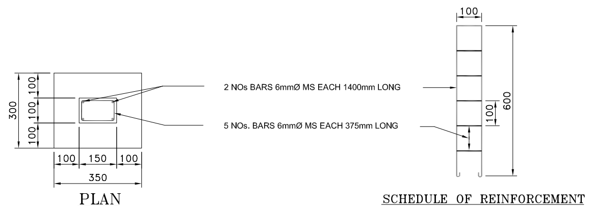
TYPE DESIGN FOR 200 - METRE STONES
