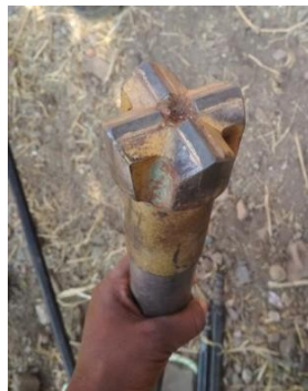
Figure 2: Drill bit for self-drilling anchors (typical cross bit)
