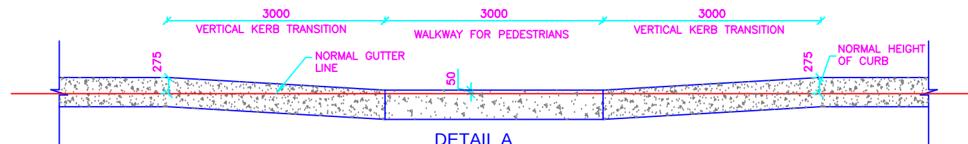
KERB DROP ON MEDIAN ALONG MAIN CARRIAGEWAY
