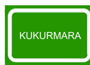
Fig. 16.06 PLACE IDENTIFICATION SIGN
