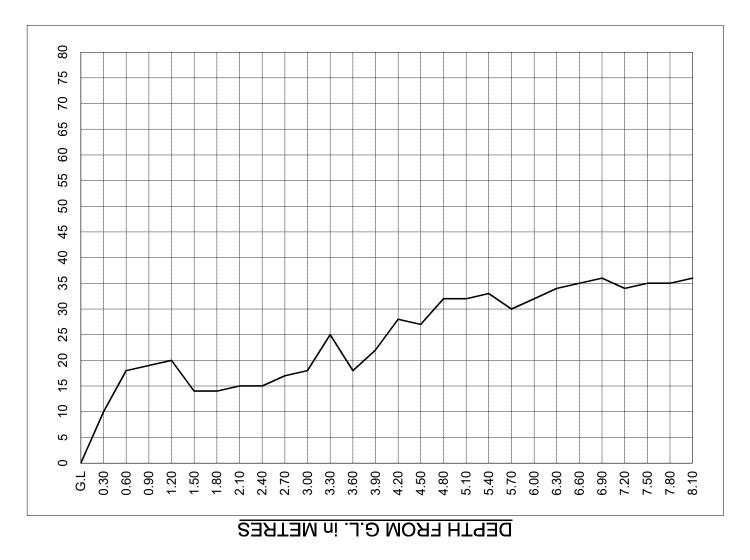
DYNAMIC CONE PENETRATION RESISTANCE CURVE FOR LOCATION No. 1.
